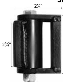
HDRBH3 3" Hinge Sealed Bearing (1.375 O.D. x .622 I.D. x .43 Thick) 4" \frac{1}{2} Bolt with nylock self-locking nut 220 Degree swing 1400 lbs/pr capacity
