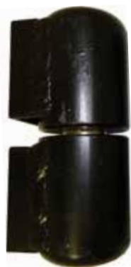
BRHS7-212 7" Steel with 1 \frac{1}{4} " SS pin 2 \frac{1}{2} " major dia. 3000 lbs/pr capacity 3/4" gap when installed
