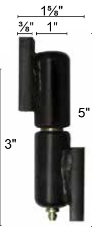
BRHS5 5" Steel with \frac{5}{8} " SS pin 1" major dia. 600 lbs/pr capacity
