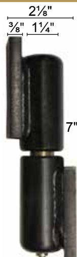
BRHS7-8 7" Steel with \frac{3}{4} " SS pin 1 \frac{1}{2} " major dia. 900 lbs/pr capacity
