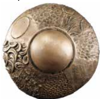
Brown Metal Oil applied to brass knob.
